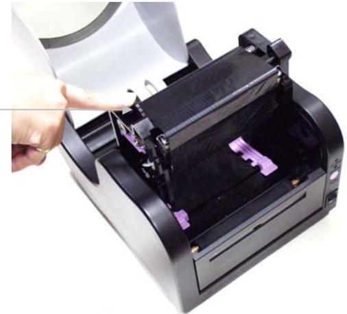
The CX400 thermal transfer printer transfers ink from a ribbon to the label to produce an image.
